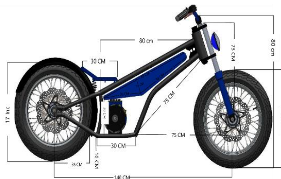
Figure 1. Conceptual design of the electric vehicle.
